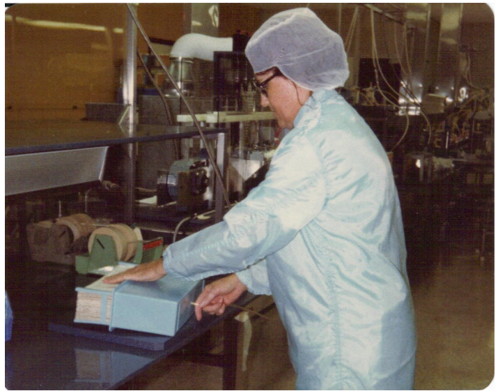
Figure 5. A worker at the Travenol plant in Hays, Kansas inserts a shim tube into a TMO membrane oxygenator (circa 1979).
