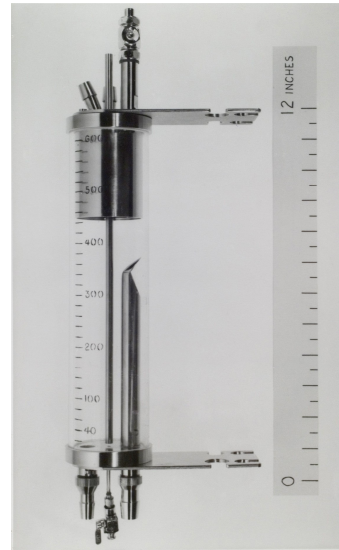
Figure 4. The venous reservoir (600 ml). Venous blood entered at the bottom and cardiectomy blood through the antifoam coated stainless steel mesh at the top.
