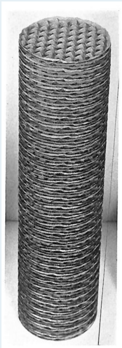
Figure 1. Stedman Packing discs used for gas exchange in Bailey's film oxygenator (photo reprinted with permission from Elsevier Publishing).
