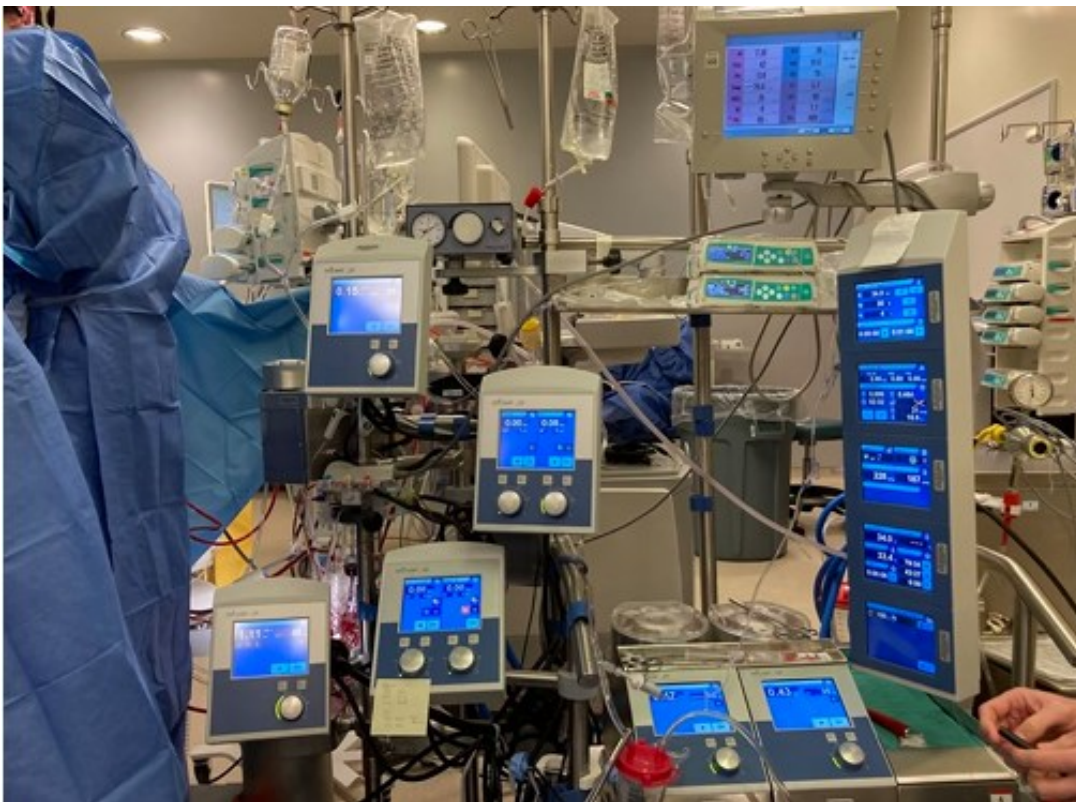
The Infant Paediatric Sorin Heart Lung machine with its modular base design, during clinical use with the Sorin Infant FX05 Hollow Fibre Oxygenator, IWK Hospital, Halifax, January 2022 (🙏).
